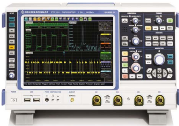
Figure 1 Rohde & Schwarz has jumped into the oscilloscope market with its RTO models, which come in two- and four-channel versions with bandwidths of 1 and 2 GHz. The units’ sampling rate is 10G samples/sec. The instruments support a Windows-driven touchscreen user interface.
