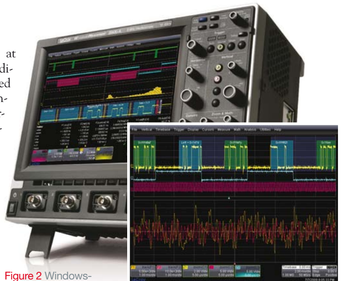
Figure 2 Windows-based oscilloscopes, such as LeCroy’s 2-GHz WaveRunner (left), can accommodate serial-data packages that support ARINC 429, MIPI, I 2 C, SPI, UART, RS-232, CAN, LIN, FlexRay, and AudioBus interfaces. LeCroy’s new measurement-and-graphing package (right) displays the left- and right-channel data from a digital-audio source that has undergone conversion into corresponding analog values and plotting over time to represent the converted analog-audio waveform. The example is from a Pink Floyd audio track and represents about a half-second of audio.
